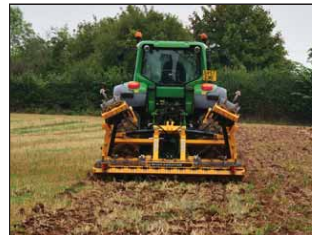
» Use as 3.0m Machine with Hydraulic Wings Raised
